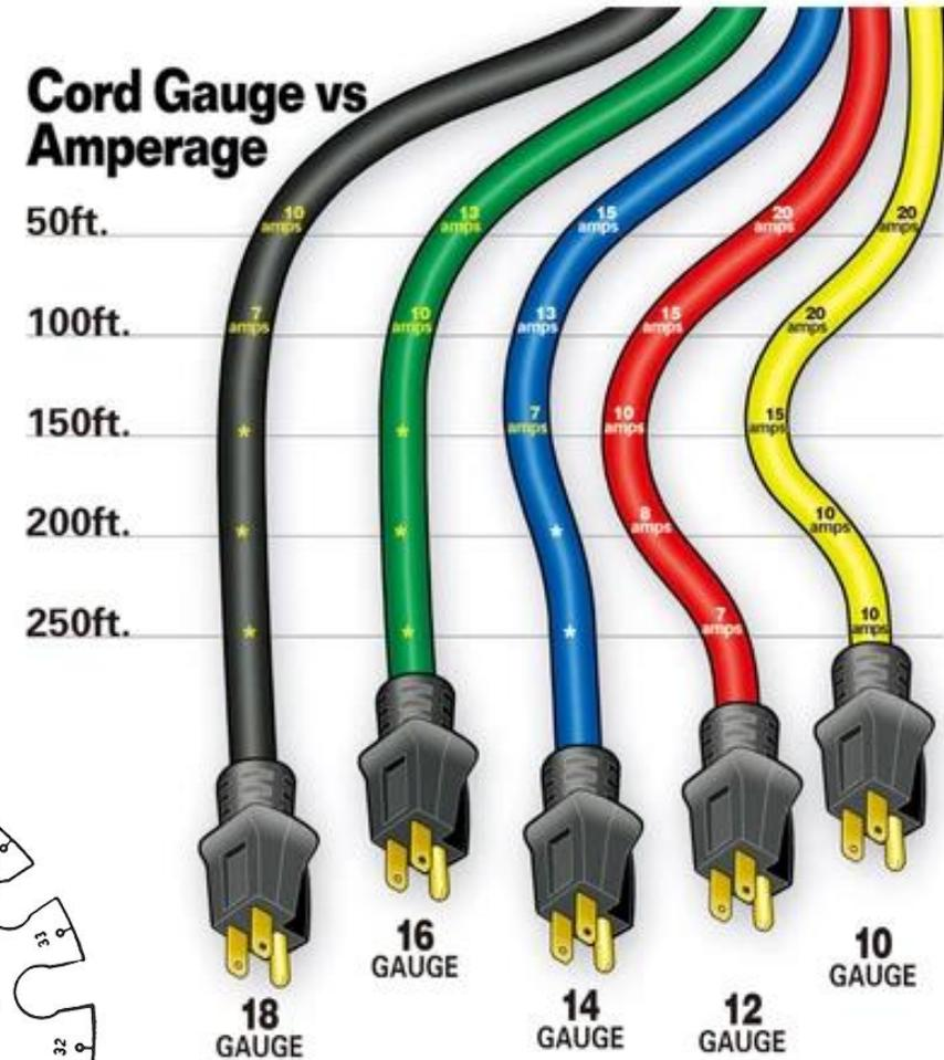
*Wire gauge measures wires ranging in size from number 36 to 0 American wire gauge (AWG)*
