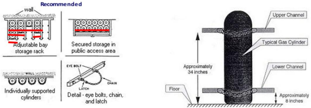
**Each cylinder must be individually secured with two restraints**
